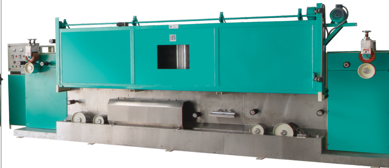
WINDER FOR FULLY AUTO STRAP WITH SPEED, TENSION AND TORQUE CONTROLLER
